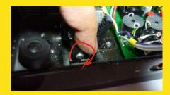
First, turn the potentiometer shaft fully counter-clockwise.
