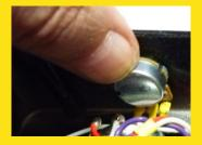
Insert the potentiometer Volume in the hole 7.5 mm and fix with nut (10mm wrench).
